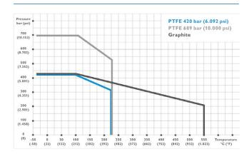
Note: All above mentioned Pressure-Temperature Ratings represent the max. allowable (Working) Pressure (PS). Note that these can be derated by the flange size or body material.
