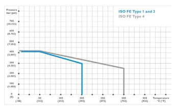
Above-mentioned Pressure-Temperature Rating is based on the standard material  $316\ \text{stainless}$  steel.
