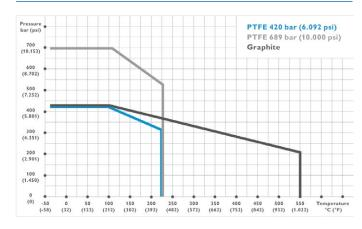
Above-mentioned Pressure-Temperature Rating is based on the standard material 316 stainless steel.
